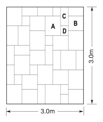
Total coverage per pack 9.0m<sup>2</sup> when laid with 7 - 14mm joints (10mm average).
